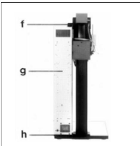
When the machine is erected, fit the holder bracket (f) to the top end of the column. Leave the screws a little loose. Put the services conduit (g) into the illustrated position, and fasten it to the bottom holder bracket (h) first. Screw the services conduit to the top holding bracket (f) as well, and tighten the two screws on the holding bracket firmly.
